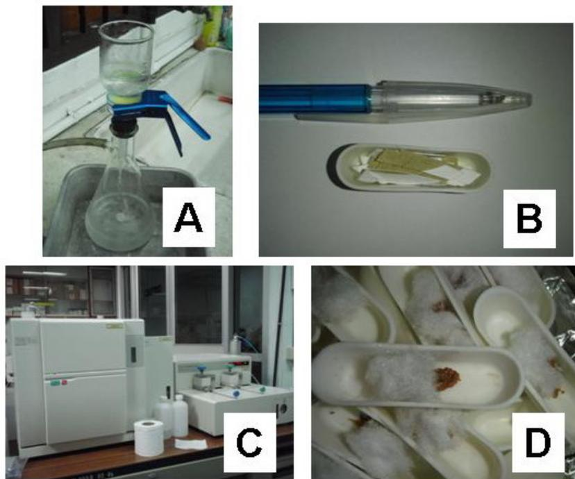
Figure 3.7 Process of POC analysis; (A) Filtering sediment, (B) Filtered filter ready to analyzed, (C) TOC analyzer and (D) Residue of filter after process
